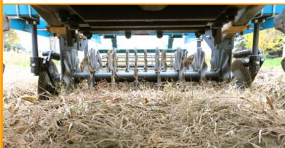
Front view of double-row coulters gangs
